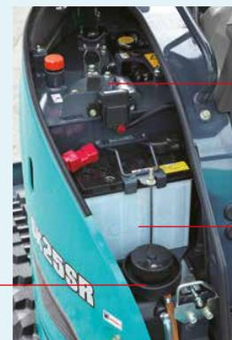
Fuel tank Hydraulic tank Battery
