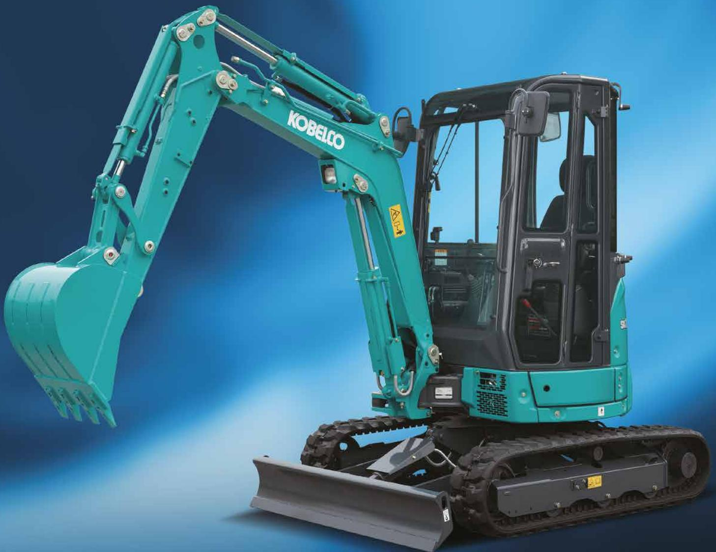
Mini excavators are widely used at sites where space is limited, such as residential areas and industrial operations. Users want big power in a small machine, stable operation, rugged construction and durability to reduce downtime. The SK25SR combines a compact design with efficiency, maneuverability and durability to ensure a long working life. Maintenance is easy, with the machine's running condition shown on an LCD monitor fitted as standard.
