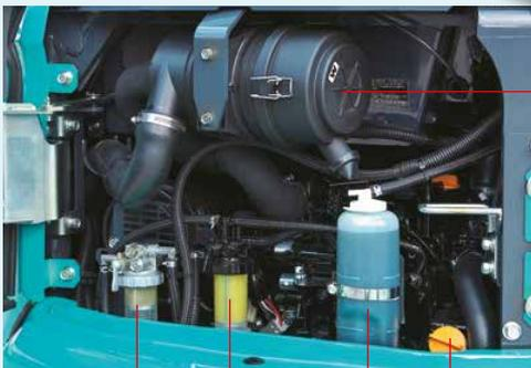
Water separator Fuel filter Radiator over flow bottle Engine oil filter
