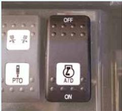
If the operating levers have been in neutral for more than 4 seconds, the engine will automatically drop back to idle, which lowers noise, emissions and fuel consumption.
