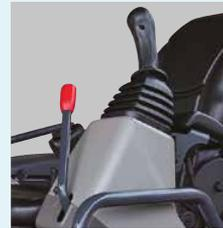
Safety lever lock permits enter and exit only when the levers are disengaged to prevent accidental operation.
