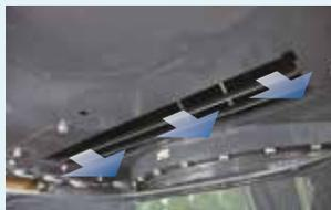
Exhaust from the muffler and engine cooling fan.
