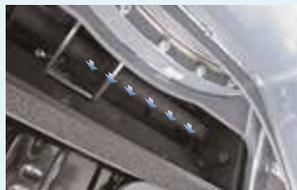
Holes on the muffler disperse exhaust
