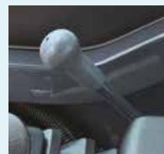
The dozer lever features hydraulic pilot control for precise handling.
