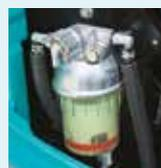
Pre fuel filter with built-in water separator
