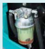
Pre fuel filter with built-in water separator
