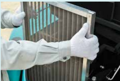
• 30-mesh means that there are 30 holes formed by horizontal and vertical wires in every square inch of filter.
