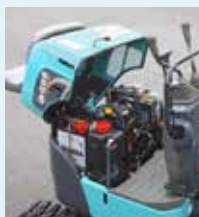
Fully opening hood for large access space.
