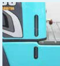
Fuel tank gauge that shows the fuel level at a glance.
