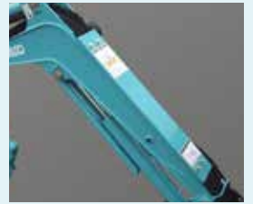
Hose protection cover on back of boom
