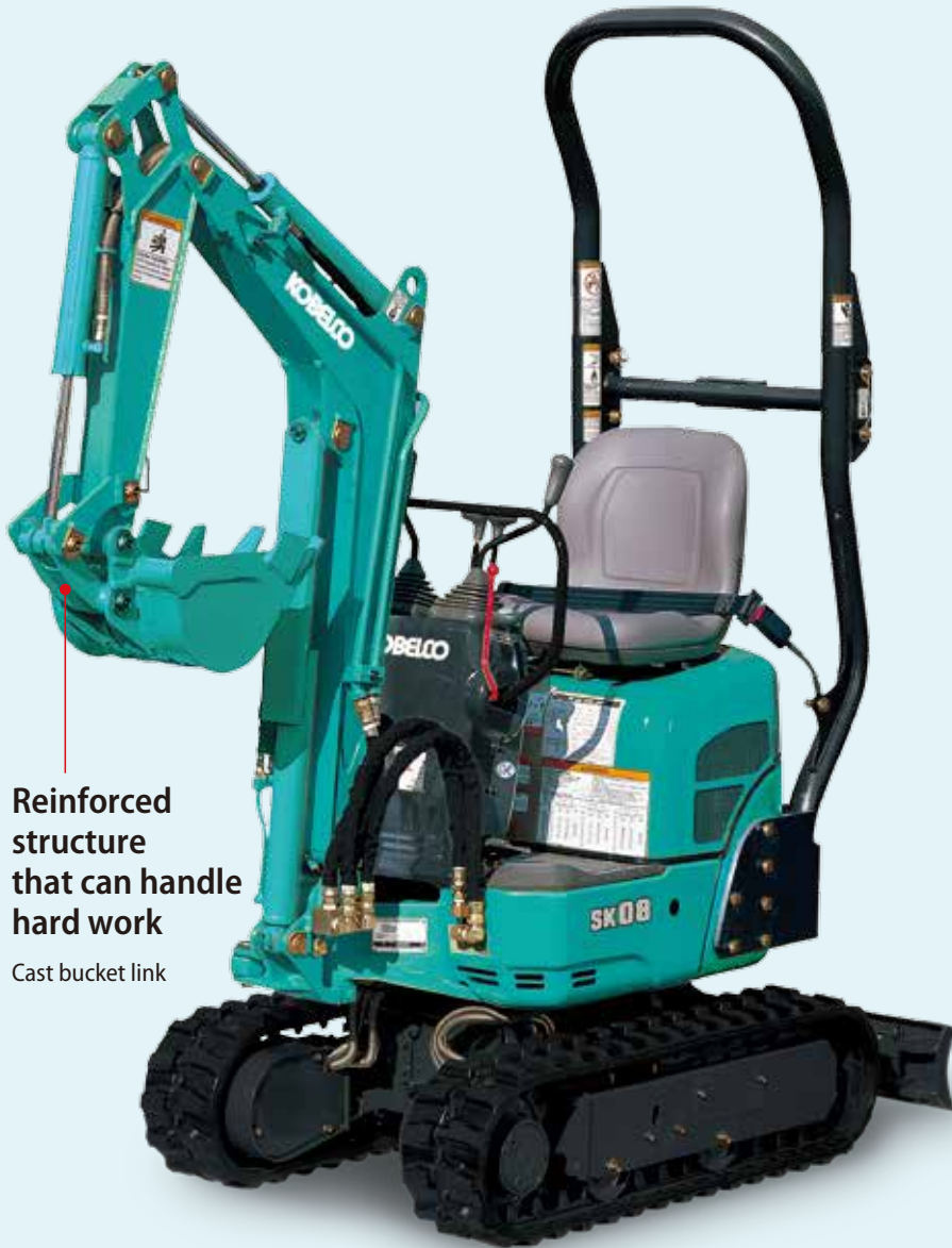
Bucket cylinder hose inside the arm
