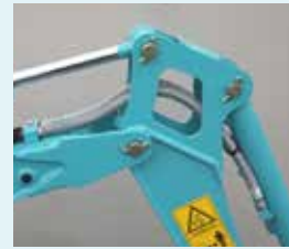
Bucket cylinder hose inside the arm
