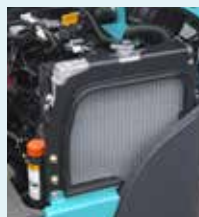
Corrosion-resistant aluminum radiator.
