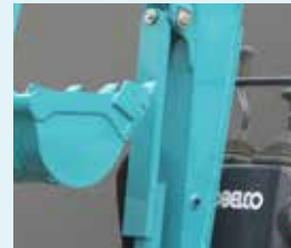
Boom cylinder protection cover
