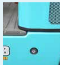
Easily checkable hydraulic oil tank gauge.
