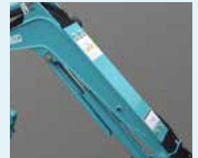
Hose protection cover on back of boom
