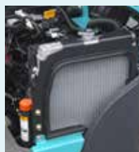
Corrosion-resistant aluminum radiator.
