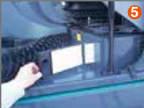
Air conditioner filter can be easily removed.
