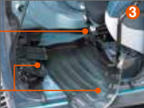
Detachable two-piece floor mat with handles for easy removal.
