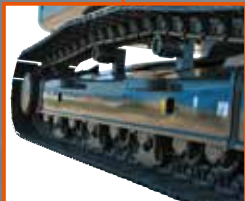
Reinforced track guides installed on three places
