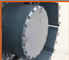
Stronger casing for travel motor
