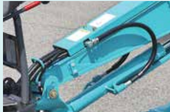
Protective cover for hoses behind the boom
