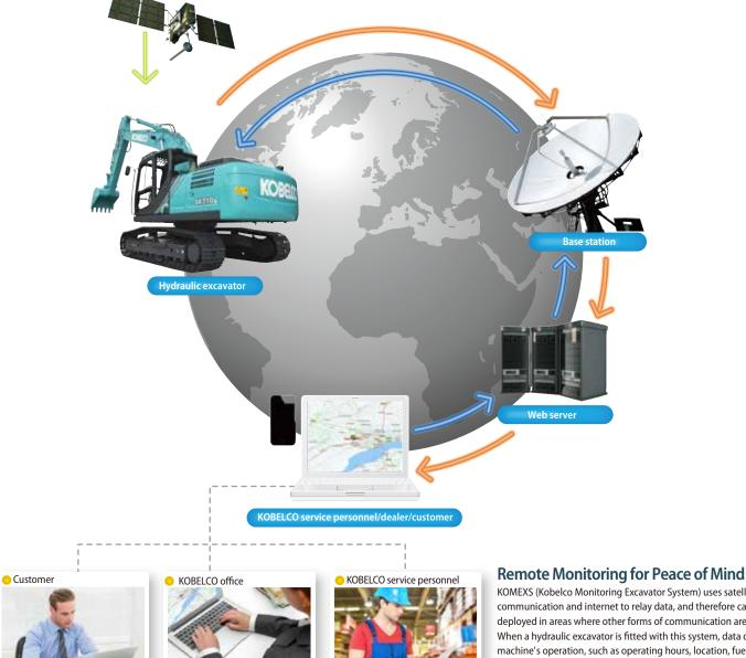
KOMEXS (Kobelco Monitoring Excavator System) uses satellite communication and internet to relay data, and therefore can be deployed in areas where other forms of communication are difficult. When a hydraulic excavator is fitted with this system, data on the machine's operation, such as operating hours, location, fuel consumption, and maintenance status can be obtained remotely.
