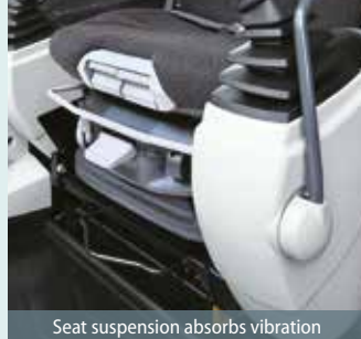
Seat suspension absorbs vibration
