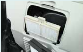
Air conditioner filter can be easily removed without tools for cleaning. One for outside air and one for inside air.
