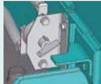
Battery disconnect switch
