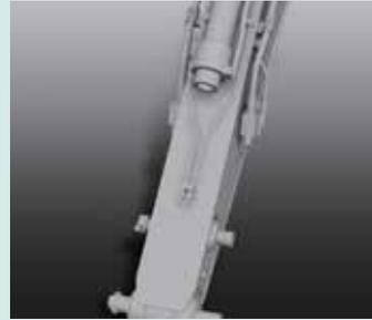
A quick hitch hydraulic line, which speeds up attachment changes, is equipped as standard.
