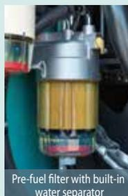
Pre-fuel filter with built-in water separator
