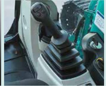
It takes 25% less effort to work the operation lever, which reduces fatigue over long working hours or continued operations.
