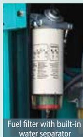
Fuel filter with built-in water separator
