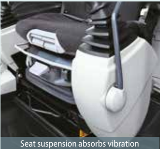
Seat suspension absorbs vibration
