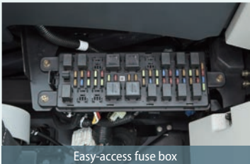
Easy-access fuse box More finely differentiated fuses make it easier to locate malfunctions.
