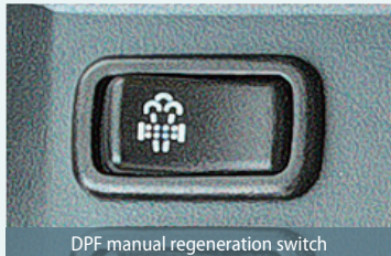
DPF manual regeneration switch If the monitor warning goes off, the filter should be reactivated manually using a switch.
