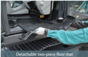
Detachable two-piece floor mat Detachable two-piece floor mat with handles for easy removal. A floor drain is located under floor mat.
