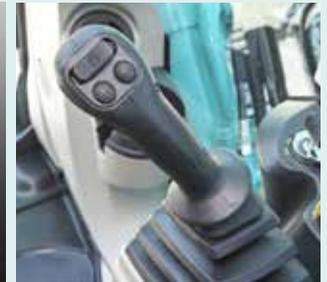
It takes 25%\* less effort to work the operation lever, which reduces fatigue over long working hours or continued operations.
