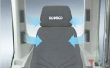
The large air-conditioner has registers on the back pillars that blow from behind and to the right and left of the operator's seat. They can be adjusted to put a direct flow of cool/warm air on the operator, which means a more comfortable operating environment.
