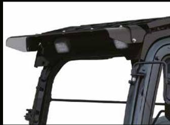
Rain visor and Cab 2 lights is fitted as optional
