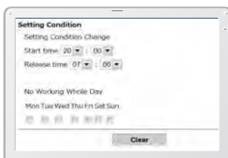
Engine start alarm outside prescribed work time
