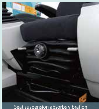
Seat suspension absorbs vibration
