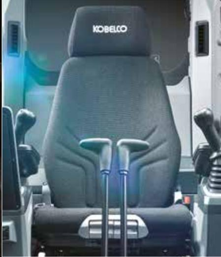
An air suspension seat manufactured by the German GRAMMER AG comes as standard equipment. It has superior shock absorption and can be used for long periods of time without causing fatigue. The included armrest is 4 inches wide.
