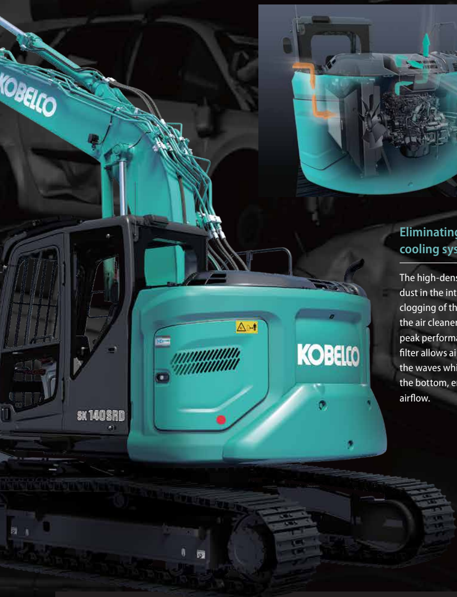
How the filter catches dust
