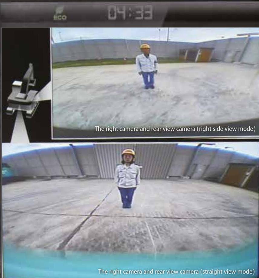
The right camera and rear view camera (right side view mode)
