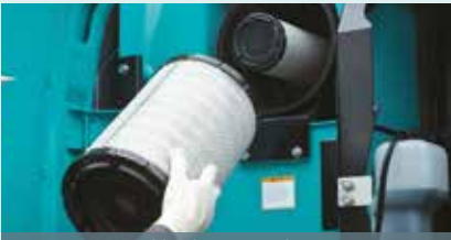
Double-element air cleaner
