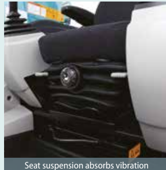
Seat suspension absorbs vibration
