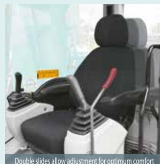
Double slides allow adjustment for optimum comfort
