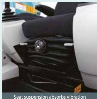
Seat suspension absorbs vibration
