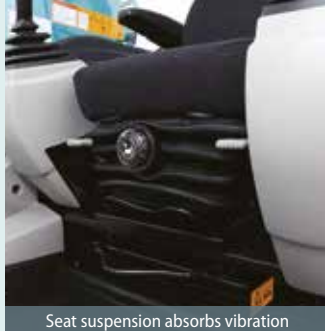
Seat suspension absorbs vibration
