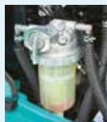
Pre fuel filter with built-in water separator
