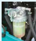
Pre fuel filter with built-in water separator
