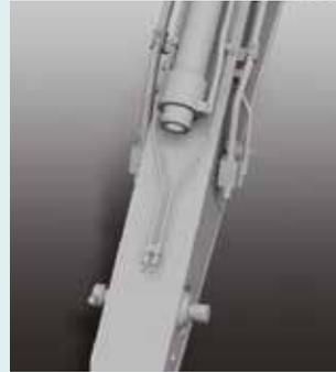
A quick hitch hydraulic line, which speeds up attachment changes, is available as an option.
