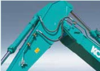
Piping for Nibbler & Breaker is fitted as standard.
