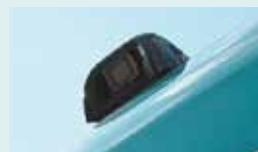
A rear view camera is installed as option to simplify checking for safety behind the machine. The picture appears on the color monitor.
