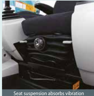
Seat suspension absorbs vibration
