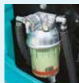
Pre fuel filter with built-in water separator
