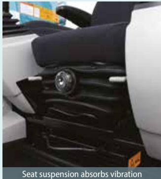
Seat suspension absorbs vibration
