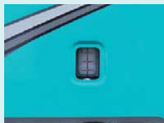
Hydraulic oil tank gauge
