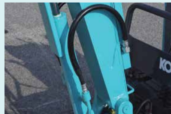
2-part type boom cylinder hoses
