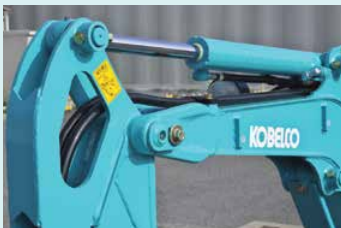
Bucket cylinder hoses sited within the arm
