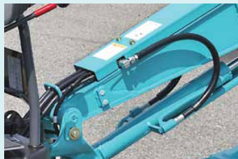
Protective cover for hoses behind the boom
