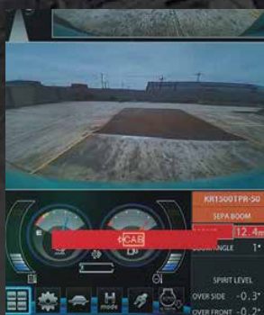
Cab interference warning display
