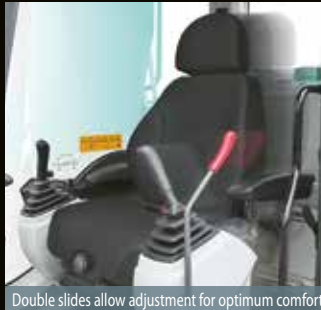
Double slides allow adjustment for optimum comfort
