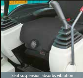
Seat suspension absorbs vibration
