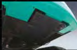
Reinforced upper frame under cover guards 6mm-thick steel plate cover protects devices in the base machine.
