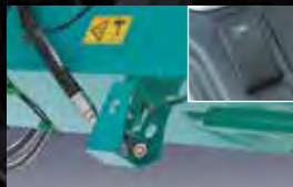
Water spray Drain circuit is provided for rust prevention.
