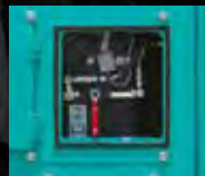
Emergency manual valve for lowering cab
