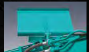
Falling object deflector The guard deflects falling debris away from the machine. This is standard for the ultra long attachment.
