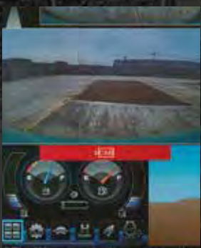
Cab interference warning display
