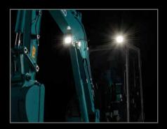
**LED work light**Changed from halogen light to LED light for more brightness.
