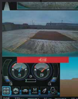
Cab interference warning display
