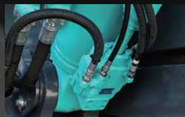
Safety valve for boom & arm & jib cylinder Prevents attachment from falling if piping is ruptured.
