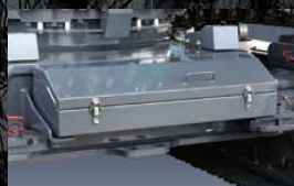
Additional storage box (option SK350DLC) Equipped with a storage box for storing tools and implements.
