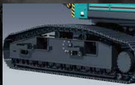
Full truck guide (option) Prevents treads from coming off when mounting on demolition rubble.
