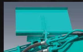
Falling object deflector (Ultra long attachment) The guard deflects falling debris away from the machine.
