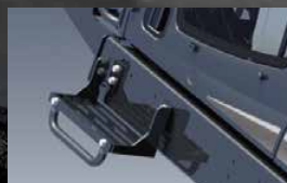
Cab entry step Positioned for convenient access to the tilt cab.
