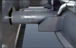
Crawler extension / retraction mechanism guard (only SK400DLC) Hydraulic cylinders protected from flying demolition debris.
