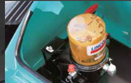
Auto lubrication system Quickly lubricate the attachments.
