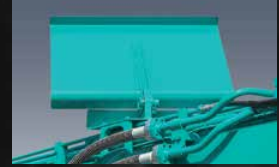
Falling object deflector (Ultra long attachment) The guard deflects falling debris away from the machine.
