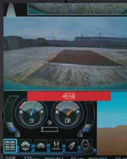
Cab interference warning display
