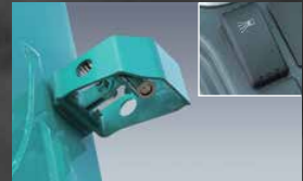
Water spray Drain circuit is provided for rust prevention.
