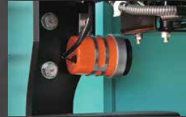
Travel alarm The alarm cautions workers in the area that the machine is traveling.
