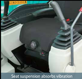
Seat suspension absorbs vibration
