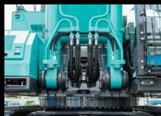
Safety valve Boom, arm and jib cylinders are equipped with safety valves for increased safety.
