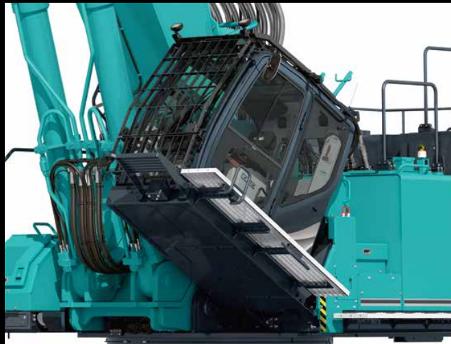
Cab can be tilted up to 30 degrees
