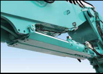
Jib cylinder guard (Only separate boom) Jib cylinder guarding is installed to prevent damage during demolition operations.
