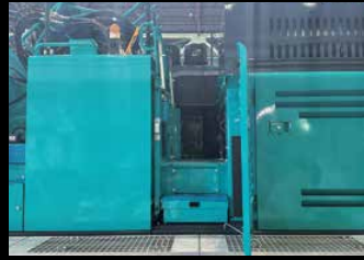
Maintenance walkway ② A walkway is provided, allowing easy access to inspection and maintenance points.
