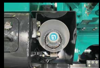
Public address system (PA system) Maintains safety by alerting workers in the area with clear audio quality.
