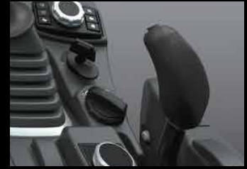
4-piece control lever The 4-piece control lever has been moved to a position that is easier to operate with grip operation.
