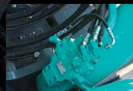
Safety valve for boom & arm & jib cylinder Prevents attachment from falling if piping is ruptured.
