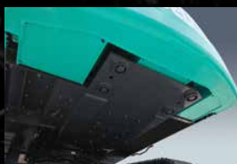
Reinforced upper frame under cover guards 6mm-thick steel plate cover protects devices in the base machine.
