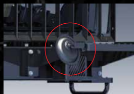
Cab lower mirror Check safety at foot areas and under the cab when tilted.
