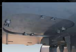
Lower frame guard 9mm-thick steel plate cover protects travel-system hydraulic circuits.
