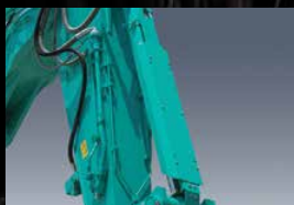
Bucket cylinder guard Prevents damage to the cylinder from falling debris.
