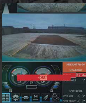
Cab interference warning display
