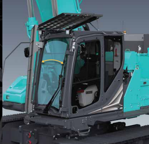
Front guard and Top guard are standard
