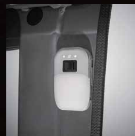
Automatic LED door light
